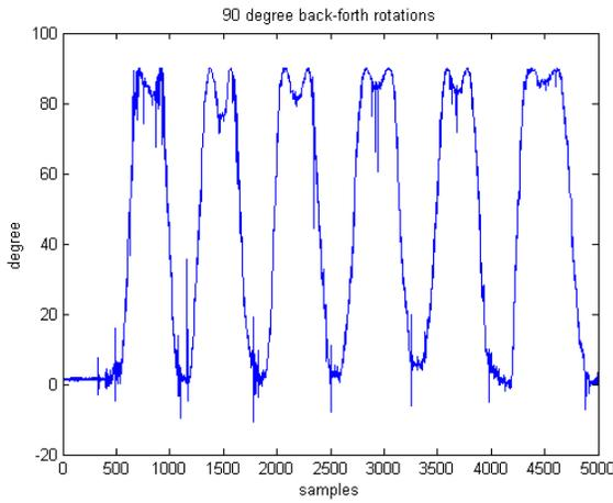
Figure 4: Noisy Rotation angle calculated by the Accelerometer
